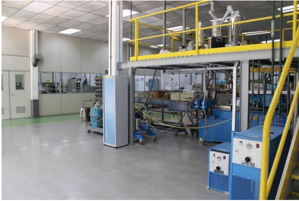
Solvay's plastics technology laboratory has an industrial scale extruder to speed up the time to market for new applications
